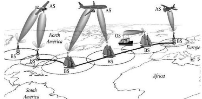
Fig.2: Airborne Internet access through stationary ships stationed along submarine optical fiber cables.
