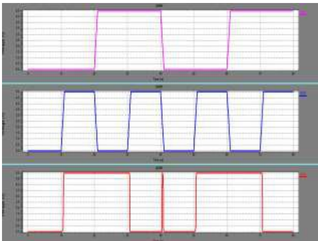
Fig. 4.2 Waveform of XOR gate
