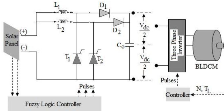
Fig.3: MPPT Based Interleaved Boost Converter Model
