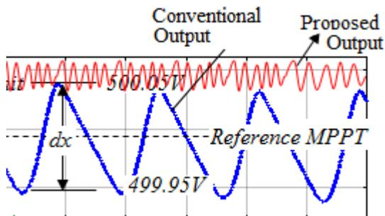
Fig.7: Effective voltage output of the proposed converter
