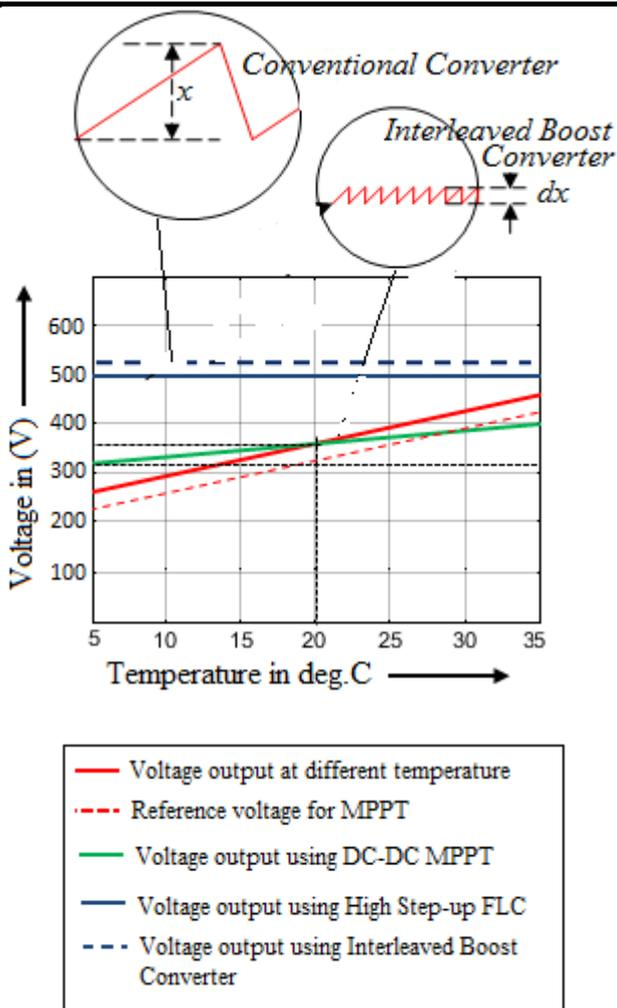
Fig.6: Voltage generated by solar panel using proposed MPPT
