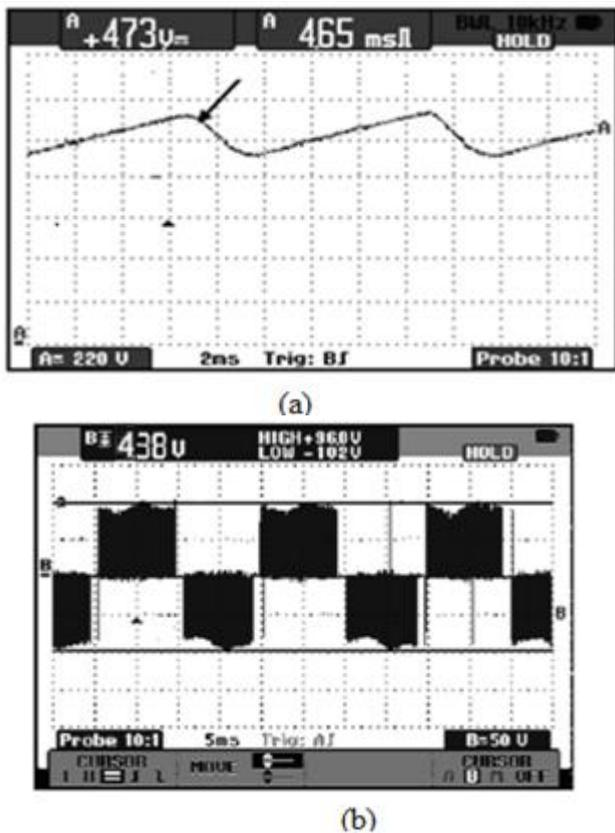
Fig.10: (a) Interleaved boost converter output (b)
