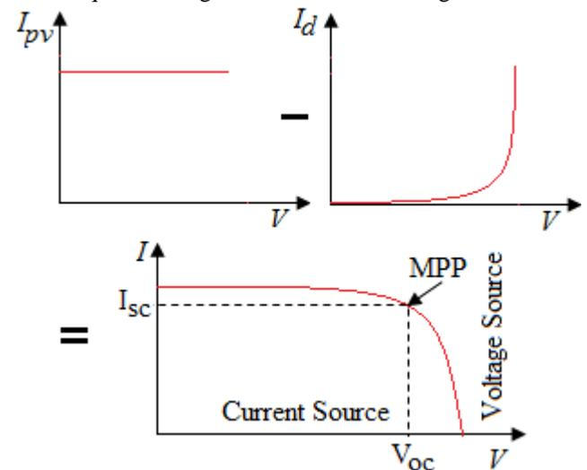
Fig.2: Origin of I-V equation of an Ideal PV cell curve of a practical PV module and Characteristic I-V curve of a practical PV module
