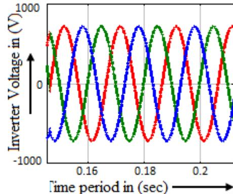
Figure 8 Three phase inverter output
